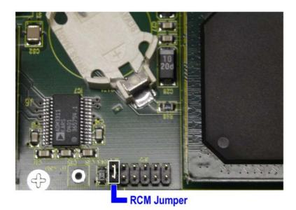
• 2. Step: Set three jumper bridges for the external LAN2 and LAN3 controller chips. The following picture shows the position.
