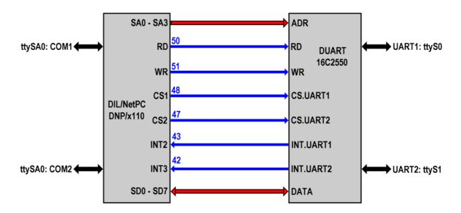
• **2. Step**: Download a Linux version with 16C2550 Dual UART support to the DNP/1110 flash memory (for example: the SSV release number 7 – 23.March.2004 – kernel version 2.4.18). The following table shows the port assignment.
