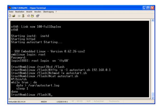
• 2. Step: Reboot the ADNP/9200. Then watch the content of the file /var/autostart.log. The Linux shell script samples file from the 1. Step writes every second a new date string into this file.
