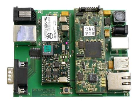
• **ISDN Modem**: The ISDN modem is the **MT128SMI-L**. The following picture shows the RAK with preinstalled MT128SMI-L modem.
