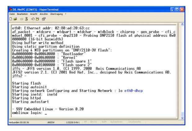
**Please note:** If DHCP doesn't work (i.e. no DHCP server available or no IP addresses available from this server), the DNP/9200 takes a default IP address. The factory-set value for this default IP address is **192.168.0.126**. The network mask for this address is **255.255.255.0**. You can change this address with an command line tool, called **ipaddree**. See *mHT9200-11.pdf: How to change the DNP/9200 Factory-Set IP Address (ipaddree usage)* for more details.
