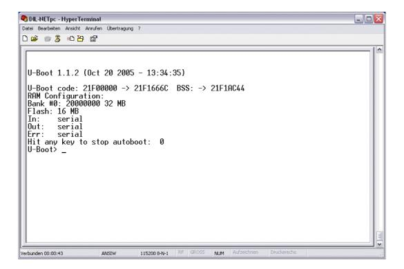
• **4. Step**: The U-Boot user interface consists of a command line interpreter (CLI), much like a Linux shell prompt. When connected via a terminal emulation program you can interactively enter commands and see the results. Please enter the **printenv** command. U-Boots shows a list of environment variables together with the current setup values.
