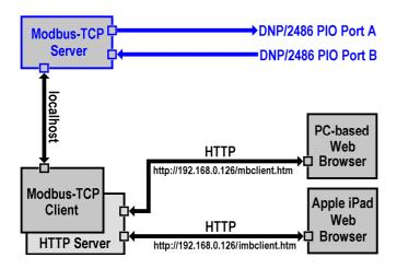
The DNP/2486 Modbus server allows Modbus-TCP-based access to the PIO Port A and Port B bits. Port A (PA0 – PA7) is used as an 8-bit output. Port B (PB0 – PB7) is used as an 8-bit input.
