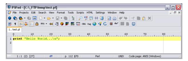
• **2. Step**: Transfer the file *test.pl* with the help of FTP or TFTP to the DIL/NetPC DNP/2486 and run the Perl script within the DNP/2486 Linux with the following command lines.
