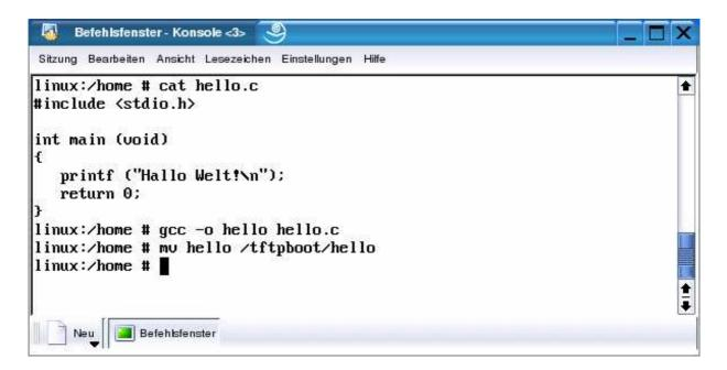
• **2. Step:** Transfer the executable with the help of FTP or TFTP to the DIL/NetPC DNP/2486 and run the executable. Don't forget the
