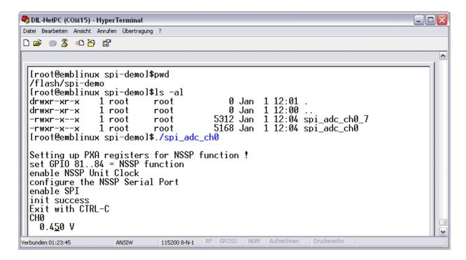
**Please note:** For a successful test please supply a voltage between 0 and 3.3 VDC to channel 0 of the SPI/ADC1 module. The SPI/ADC1 hardware reference manual describes a simple test environment. Please see this document for more details.
