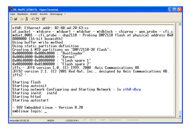
**Please note:** If DHCP doesn't work (i.e. no DHCP server available or no IP addresses available from this server), the DNP/2110 takes a default IP address. The factory-set value for this default IP address is **192.168.0.126**. The network mask for this address is **255.255.255.0**. You can change this address with an command line tool, called **ipaddree**. See *mHT2110-11.pdf*: How to change the DNP/2110 Factory-Set IP Address (ipaddree usage) for more details.
