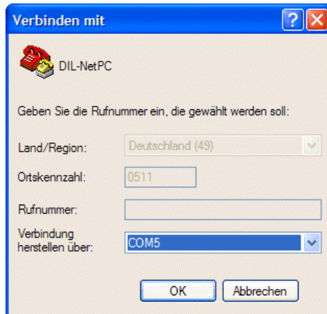
Figure 5: Direct Connection Set-up with HyperTerminal
