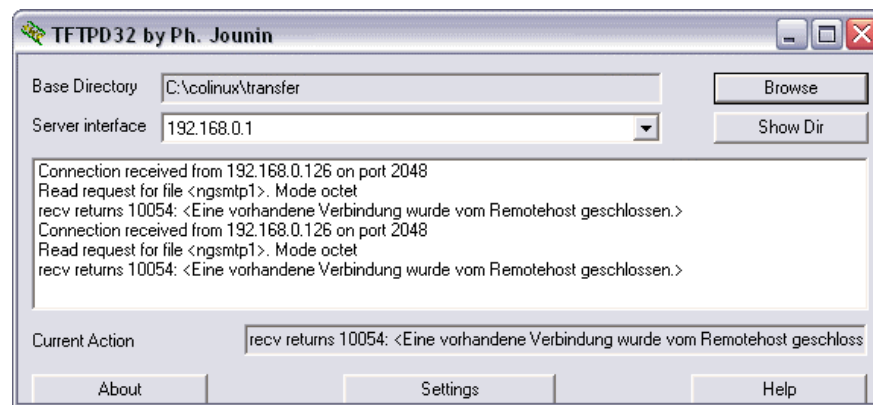
Figure 7: The TFTP server is used for file transfer
