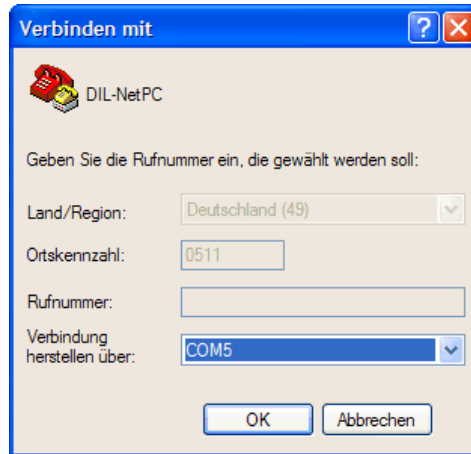
Figure 6: Direct connection setup with HyperTerminal
