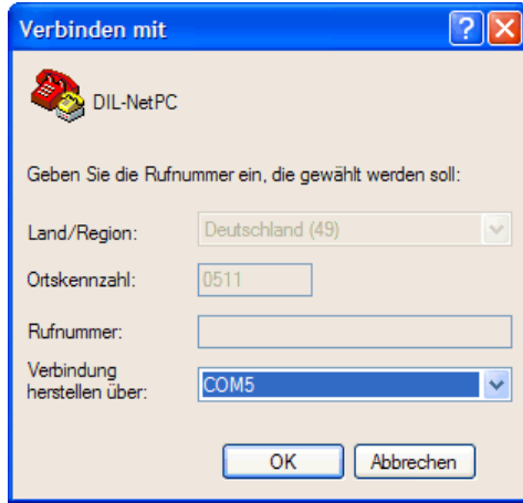
Figure 6: Direct connection setup with HyperTerminal
