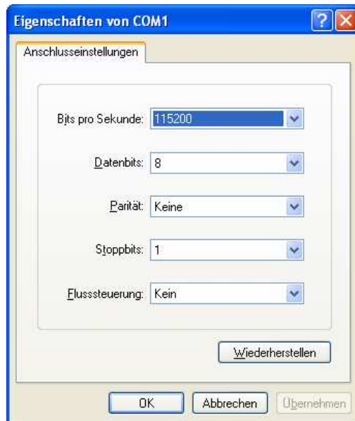
Figure 7: Parameter setup with HyperTerminal
