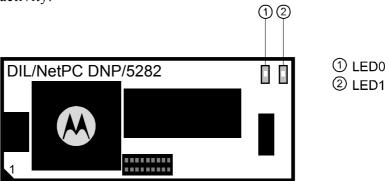
Figure 3-2: Position of the miniature LEDs on the DNP/5282
