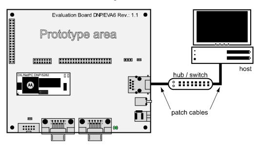
Figure 4-4: Ethernet link connection using a hub/switch
