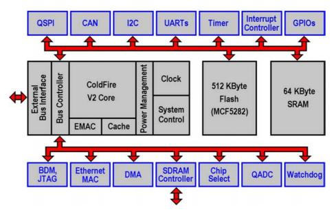
Figure A1-1: Block Diagram of the MCF5282/MCF5282-Microcontroller
