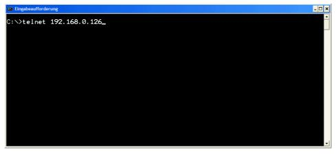
Figure 5-14: Running the MS-Windows Telnet client
