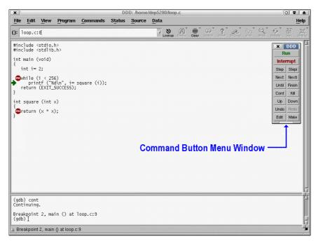
Figure 5-45: Using the command button menu window
