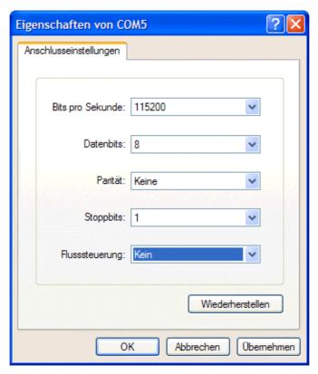
Figure 5-2: Communication parameter settings
