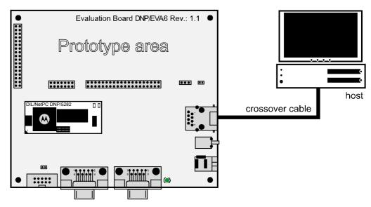
Figure 4-5: Ethernet link connection using a crossover cable
