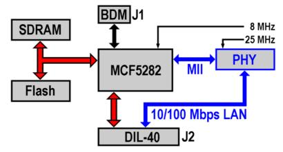
Figure A1-2: Block Diagram of the DNP/5282
