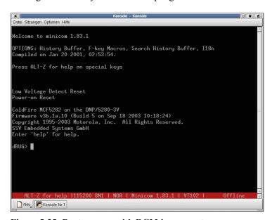
Figure 5-25: Boot process with RCM jumper set
