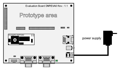
Figure 4-6: Power supply connection
