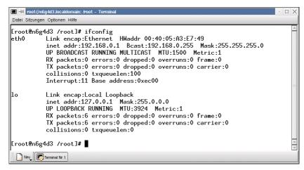
Figure 5-23: IP-address check via ifconfig
