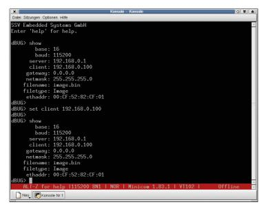
Figure 5-26: Assigning a new IP-address to the DNP/5282
