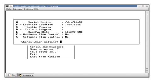
Figure 5-19: Serial port settings under Minicom
