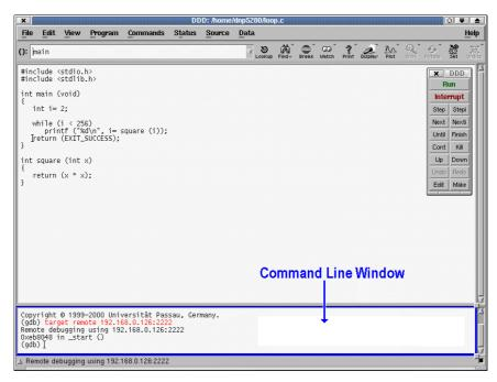
Figure 5-44: Typing commands in the command line window
