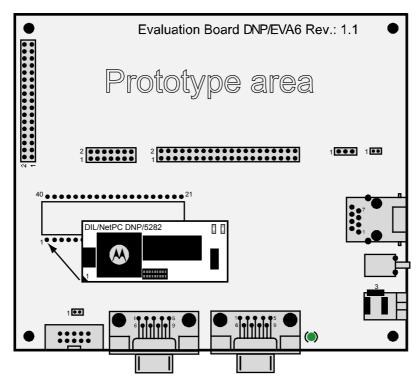
Figure 4-1: Mounting the DNP/5282 on the DNP/EVA6
