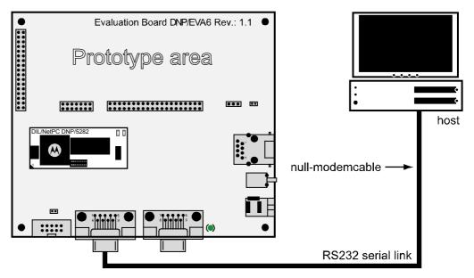
Figure 4-3: Serial link connection
