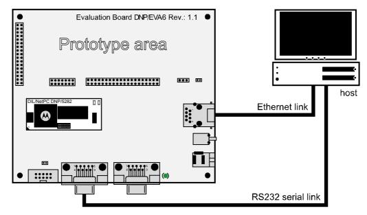
Figure 4-2: Overview about the required cable connections
