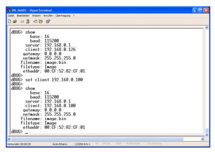
Figure 5-11: Assigning a new IP-address to the DNP/5282
