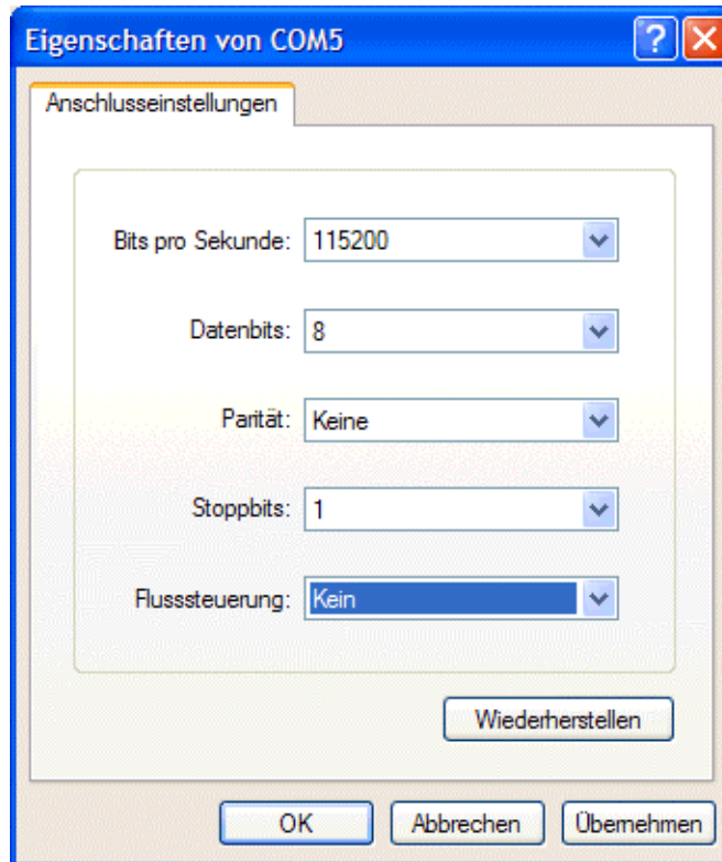
Figure 5-2: Communication parameter settings
