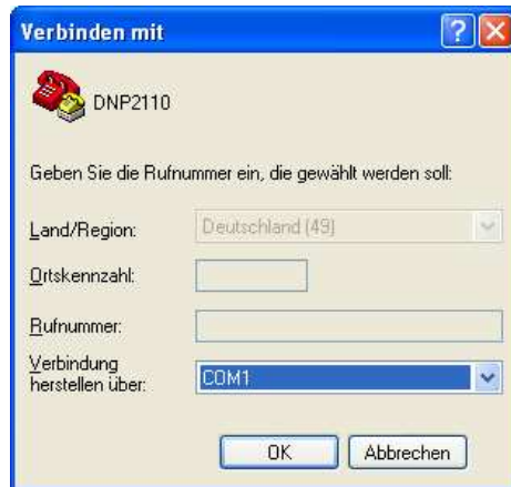
Figure 4: Direct connection setup with HyperTerminal
