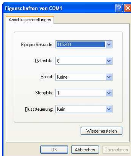
Figure 5: Parameter setup with HyperTerminal
