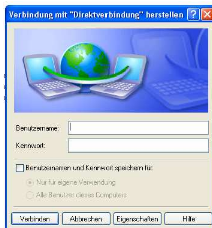
Figure 22: Starting the PPP connection on the Windows PC
